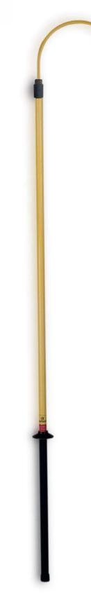
Rescue pole with only one section made of polyester and fibreglass tube  $\emptyset$  32 mm with humidity-proof seals on each end, hand protector, grip, tip, M-10 metric head and rescue hook.
